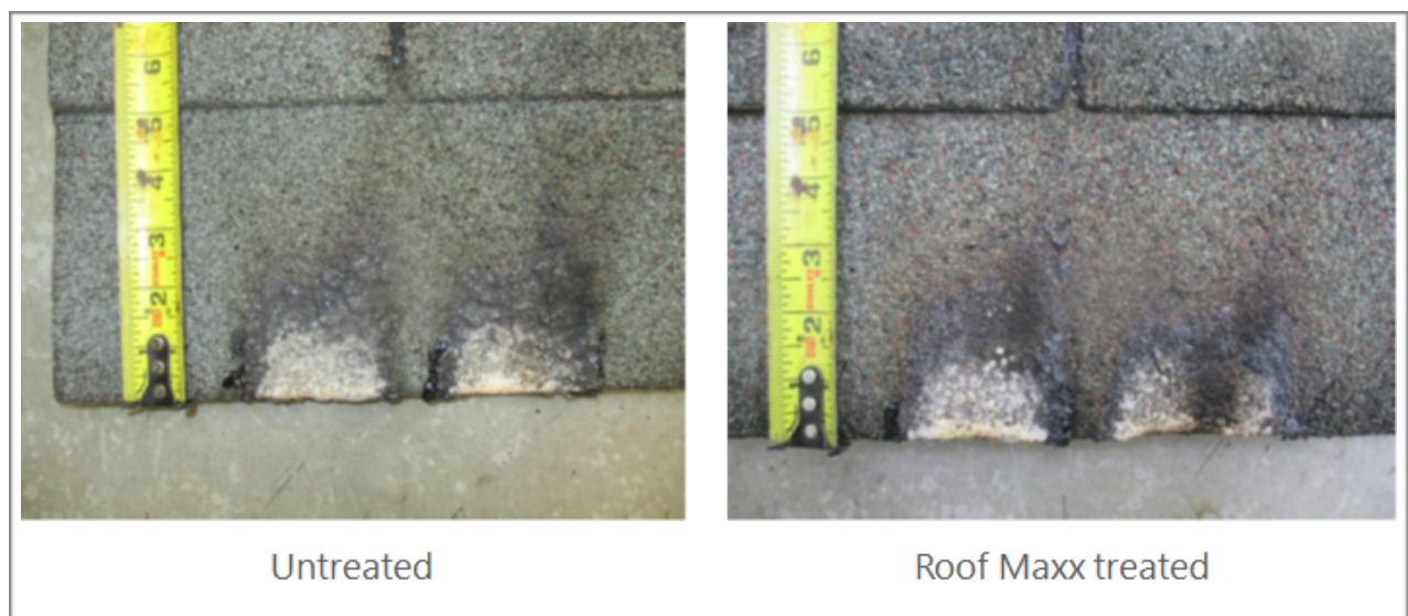
Figure 3. Spread of flame in decks of untreated and Roof Maxx treated asphalt shingles
